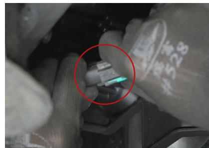
5. Plug the SS3 into the factory fog light harness using the included Molex wire adapter.
