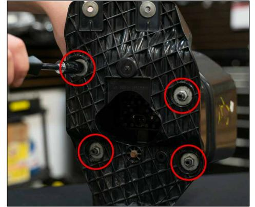
9. Reattach the front bezel using the four 13mm nuts. **Do not over tighten.**
