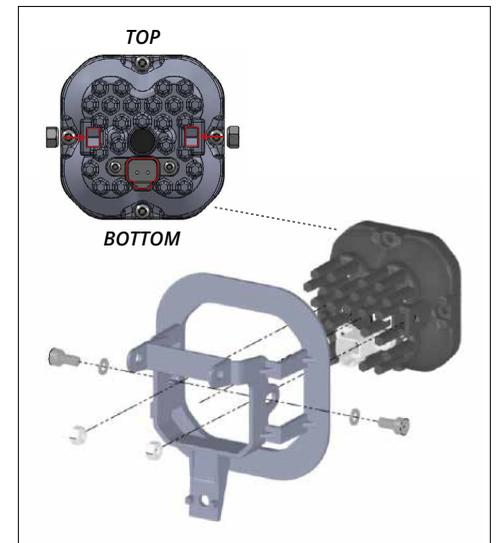
**6.** Using the included hardware, attach the Type SD bracket to the pod. See the diagram above and make sure the bracket is in the correct orientation. Tighten these bolts down all the way.
