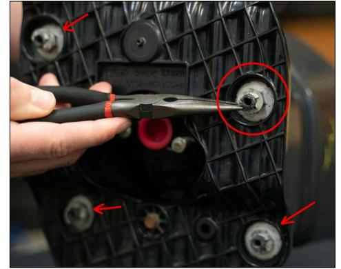
**3.** Set the foglight bracket assembly on a table. Remove the four metal retaining washers using a pick or flathead screw driver. Then remove the four 13mm nuts that secure the front bezel to the foglight bracket.
