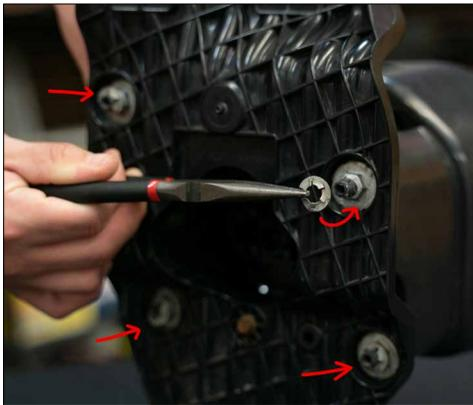
10. Reattach the metal retaining washers.
