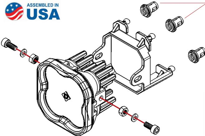
**Factory Fog Lamp Assembly Retainer Clips**
