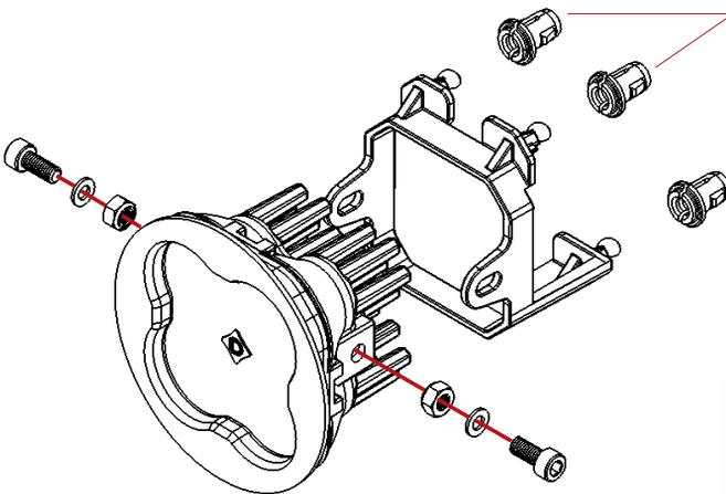
**Factory Fog Lamp Assembly Retainer Clips**
