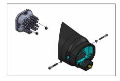
**8.** With nuts installed, place the SS3 into the bracket and bezel assembly, aligning the holes on each side.
