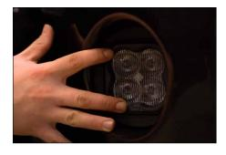
**9.** Reinstall the fog light bezel and SS3 assembly onto the vehicle, using the original hardware.
