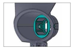
**5.** Install the SS3 bracket on to the factory bezel. Flex the outer clips of the factory bezel slightly if required.
