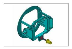
**4.** Unscrew the ball-head adjustment screw from your factory fog lamp. Remove the plastic nut from it (shown in yellow on diagram). Remove the metal clip-nut (shown in red on diagram).
