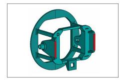
**4.** Place the rectangular adhesive pads on the back of the bracket, on each side. Adhesive pads are shown in red color on diagram above.
