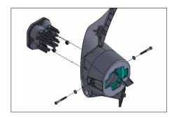
**7.** With nuts installed, place the SS3 into the bracket and bezel assembly, aligning the holes on each side.
