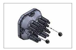
**6.** Place the supplied nuts into the holders on the SS3 pod, with the nylon locking feature facing inwards.
