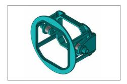
**3.** Place the included plastic spacers just inside the outer tabs of the SS3 bracket, on each side. Spacers are shown in grey color in diagram above.
