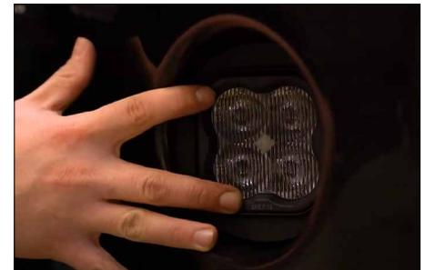
9. Reinstall the fog light bezel and SS3 assembly onto the vehicle, using the original hardware.
