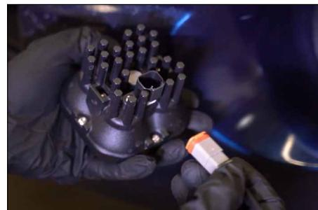
7. Place the supplied nuts into the holders on the SS3 pod, with the nylon locking feature facing inwards.
