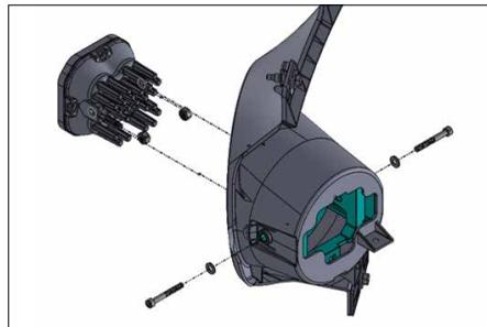
7. With nuts installed, place the SS3 into the bracket and bezel pod, aligning the holes on each side.
