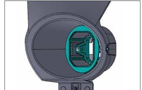
5. Install the SS3 bracket on to the factory bezel. Flex the outer clips of the factory bezel slightly if required.
