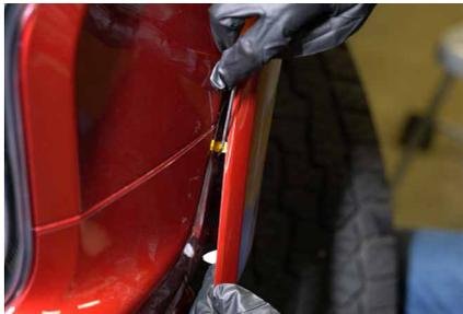
3. Peel the plastic fender flare back using a plastic trim removal tool. Loosen the plastic clips holding it in place using a pick tool.
