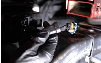
10. Reinstall the factory fog light bezel, by reinstalling the factory hardware. Plug the SS3 into the factory fog light harness using the included DT wire adapter. Test function. If the light does not turn on, try flipping the connector 180°.
