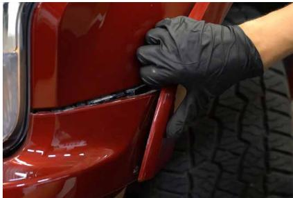
4. Using a plastic trim removal tool, loosen the upper bumper piece. Repeat the steps on the other side of the vehicle to remove the upper bumper piece from the vehicle.
