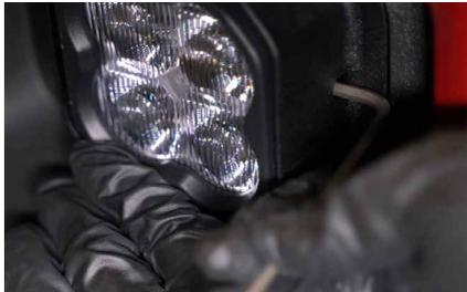
11. Adjust and aim the fog light according to your local and state laws. To adjust, loosen the screws on the sides of the bracket, aim, and re-tighten. In general, fog lamps should be angled slightly downwards to illuminate the area directly in front of the vehicle, below your headlamps.
