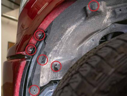
2. Peel back the wheel well fender liner. To do so, remove the two push clips, two 5.5mm bolts, and two 7mm bolts shown in the picture to the left and peel the fender liner back.
