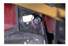
7. Remove the final 8mm bolt and loosen the plastic retaining clip to remove the fog light bezel from the vehicle.
