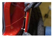
3. Peel the plastic fender flare back using a plastic trim removal tool. Loosen the plastic clips holding it in place using a pick tool.
