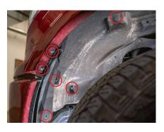
2. Peel back the wheel well fender liner. To do so. remove the two push clips, two 5.5mm bolts, and two 7mm bolts shown in the picture to the left and peel the fender liner back.
