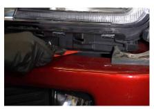
5. Remove the shroud blocking access to the fog light bezel. To do so, remove the 10mm bolt and loosen the three plastic pins holding the shroud to the bottom of the headlight. Then remove the two 10mm bolts near the fender flare. Remove the shroud from the vehicle.
