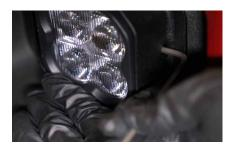
11. Adjust and aim the fog light according to your local and state laws. To adjust, loosen the screws on the sides of the bracket, aim, and re-tighten. In general, fog lamps should be angled slightly downwards to illuminate the area directly in front of the vehicle, below your headlamps.
