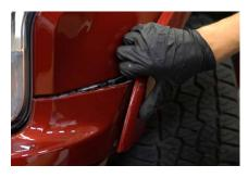
4. Using a plastic trim removal tool, loosen the upper bumper piece. Repeat the steps on the other side of the vehicle to remove the upper bumper piece from the vehicle.
