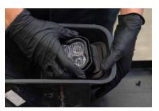
9. Install the SS3 bracket on to the factory bezel by flexing the retainer clips on the bezel as required.
