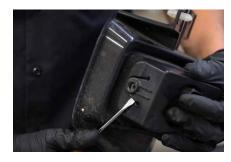
8. Remove the fog light housing from the bezel. To do so, remove the adjustment screw and spring from the fog light housing. Remove the factory fog light housing by prying up on the retainer clips holding it in place.
