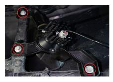
3. Install your assembled bracket and pod onto the vehicle by securing the three OEM bolts with a 10mm socket and ratchet.
