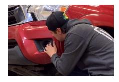
7. Loosen the 5/32" allen bolts on each side of your SS3 pod, just enough to allow you to adjust the pod.
