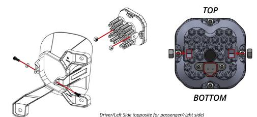
1. Install the supplied nuts into the pod housing with the nylon facing inward. Attach the bracket to the pod using the supplied screws and washers. Make sure the bracket is in the correct orientation. See diagrams above. Ensure that the screws are tightened such that the pod retains its position, but can pivot with force for aiming.
