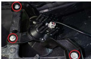
3. Install your assembled bracket and pod onto the vehicle by securing the three OEM bolts with a 10mm socket and ratchet.
