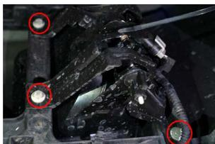
2. Access your factory fog lights and unplug the fog lamp connector. Use a 10mm socket and ratchet to remove the three bolts, as shown in the picture to the left. Remove the factory fog light housing. The factory bolts will be reused.
