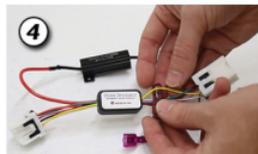
Before installing your Diode Dynamics module, apply the included t-tap to the yellow back up light wire and ensure it makes a proper connection by using pliers to clamp it down.
