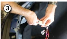
Take your Diode Dynamics module and plug it in inline. Then replace the carpet and repeat for the other side.
