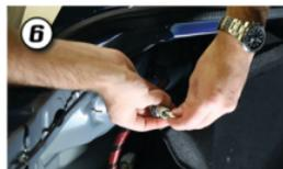
Next, remove the 2 locking screws holding the carpet in place to give you more room to work. Install the module inline on each side of the vehicle. Replace your factory turn signal bulb with a white LED bulb by pulling the rubber cover off and turning the socket counter-clockwise to remove it.
