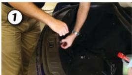
Using a small flat head screwdriver or trim tool, remove the 5 locking screws holding the center trim piece in place. Pull the trim piece straight up to remove it and set it aside.
