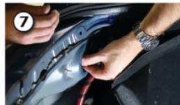
Once the new bulb is installed, lock the socket back in place by turning clockwise and replacing the rubber cover. Repeat the same process for your factory back-up bulb. Then repeat for both bulbs on the other side of the vehicle.
