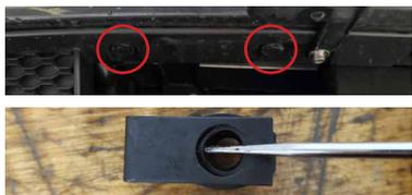
4. Install the four included clip-on barrel nuts in the holes along the top of the lower grille where the push rivets were previously located.
