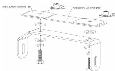
5. Using a 13mm socket and the included M8 bolts, washers, and lock washers, install your new light bar brackets as shown to the left.
