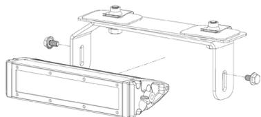
7. Using a 10mm wrench and the included hardware, install the light bars onto the brackets. Using the adjustment slots, adjust the height of the light bars, and adjust the brackets so that light is being directed where desired. Once adjustments are complete, tighten the 10mm and 13mm nuts.
