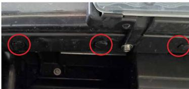
2. Using a trim removal tool or flat-head screwdriver, remove the five plastic push-rivets from along the top of the lower grille opening.
