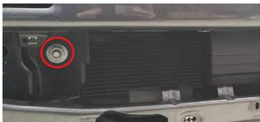
6. Remove the two 21mm frame nuts shown in the picture to the left on each side of the vehicle.
