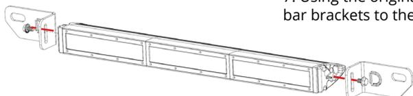
7. Using the original 21mm nuts, install your new light bar brackets to the studs, hand-tightening them only.
