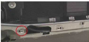
9. Reinstall the lower grille and license plate holder (if applicable) using the original hardware. Ensure the mounting clips shown in the image to the left are properly bent such that they will not push through the sheet metal backing, that the mounting clip ribs are pointing rearward such that the plastic panel can be inserted with minimal interference.
