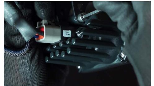
15. Aim the pods as desired. Then tighten down the hardware using a 5/32" allen-key and a 3/8" wrench. Aiming can be achieved with the pods installed on the vehicle. There is no need to remove the pods to re-aim.
