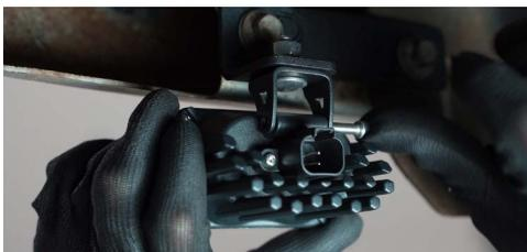
4. Install your new SSC1 or SSC2 pod onto the universal pod bracket using the provided hardware. Using a 5/32" allen-key and a 3/8" wrench, tighten the screw such that the pod retains its position, but can pivot with force for aiming.
