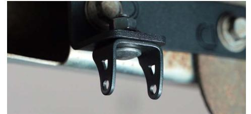
3. Install the universal pod bracket onto the reverse light bracket using the provided hardware. Make sure that the curved portion of the bracket is facing towards the rear of the vehicle.
