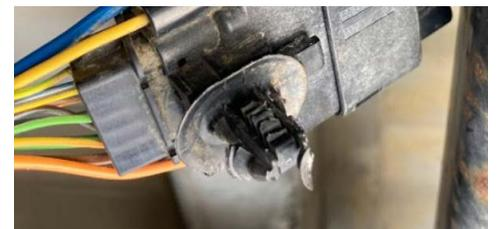
6. Using a plastic rivet removal tool, free the connector from the vehicle.
