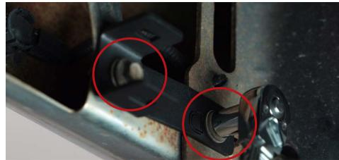
2. Install your new reverse light bracket onto the vehicle using the factory bolts removed in the previous step.
