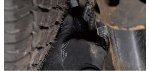
9. Reinstall the Molex (Type A) connector to the vehicle and secure it using the plastic rivet.
