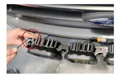
14. With all three 10mm bolts tightened down, adjust the gap on the opposite side pivot mount and secure the mount using the 5mm Allen wrench.
