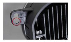
**TOYOTA VEHICLES:** While installing the lamp, flex the left side tabs outward to insert them into the mounting pockets. Use the bottom portion of the slot on the bracket to secure the factory screw (shown in red in picture to the left).
