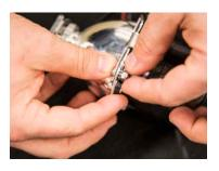
2. Next, mount the Demon Eye inside the projector housing, ensuring the Demon Eye board is inside the shroud. The bracket can be mounted on either the front or the back side of the projector housing. Using the mounting holes and included locking screws, secure both sides of the bracket to the housing. Again, thread the locking screws and locknuts and then tighten using pliers and a small Philips screwdriver.
