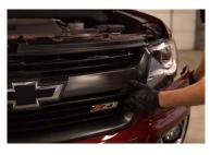
6. Remove the bumper and grille by pulling straight out from the vehicle and releasing the two push tabs securing the bumper to the front of the vehicle. Set the bumper and grille aside on a soft surface.
