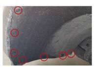
1. Remove the six T15 torx screws from the wheel well holding the fender liner in place. With the fender liner pulled back, remove the 7mm hex bolt from the bumper support, holding the bumper to the chassis.
