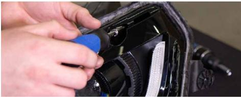
1. Remove the six T20 torx screws holding the black bezel in place, including the screw on the backside of the housing. Set the bezel aside.
