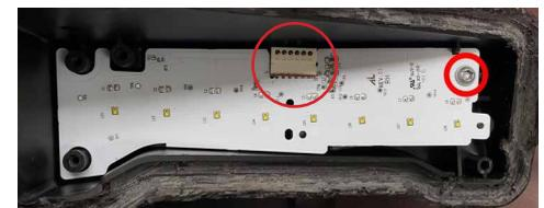
10. Remove the single T25 torx screw from the factory board. Then remove the factory board and disconnect the OEM connector. It won't be reused.
