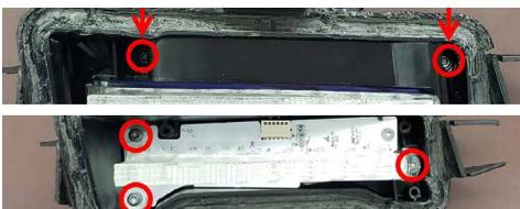
8. Remove the two T25 torx screws holding the black plastic shroud in place.
