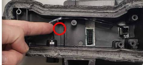
12. Drill a hole just large enough for your new wiring harness to pass through. You may need to de-pin the connector and re-pin after passing through for a proper seal.
