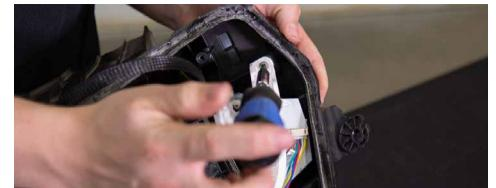
6. Using the original T20 screws, reinstall the white optics shroud and route the wires through the back of the headlight assembly, sealing any holes you may create.
