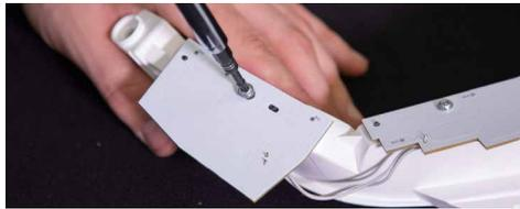
2. Remove the four T10 torx screws holding the factory boards in place. Then remove the factory boards. They won't be reused.
