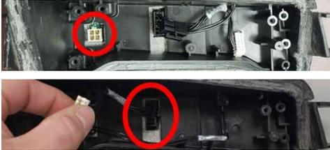
11. Disconnect the OEM driver harness from the driver and remove the harness from the lamp.
