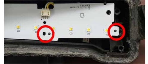
13. Install your new LED board into the lamp housing, aligning the tabs. Then reinstall the original screws and optic. Reinstall the black shroud. Once complete, repeat the same process for the other lamp.
