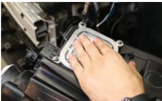
2. Remove the bumper and headlamp from the vehicle. Next, mount the demon eye in the headlamp. To do so, remove the 4 screws holding the HID ballast in place using a T20 Torx bit.
