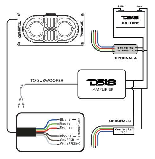
Black Wire "BK" Connected to Battery Positive (+12v) Blue Color Light "B" Connected to Battery Negative (-) Green Color Light "G" Connected to Battery Negative (-) Red Color Light "R" Connected to Battery Negative (-) Purple Color Light "R" and "B" Connected to Battery Negative (-) Yellow Color Light "R" and "G" Connected to Battery Negative (-) Cyan Color Light "B" and "G" Connected to Battery Negative (-) White Color Light "R"; "B" and "G" Connected to Battery Negative (-)
