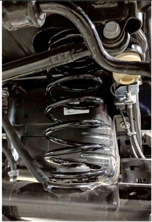
Figure 1. Correctly Installed Rear Spring
