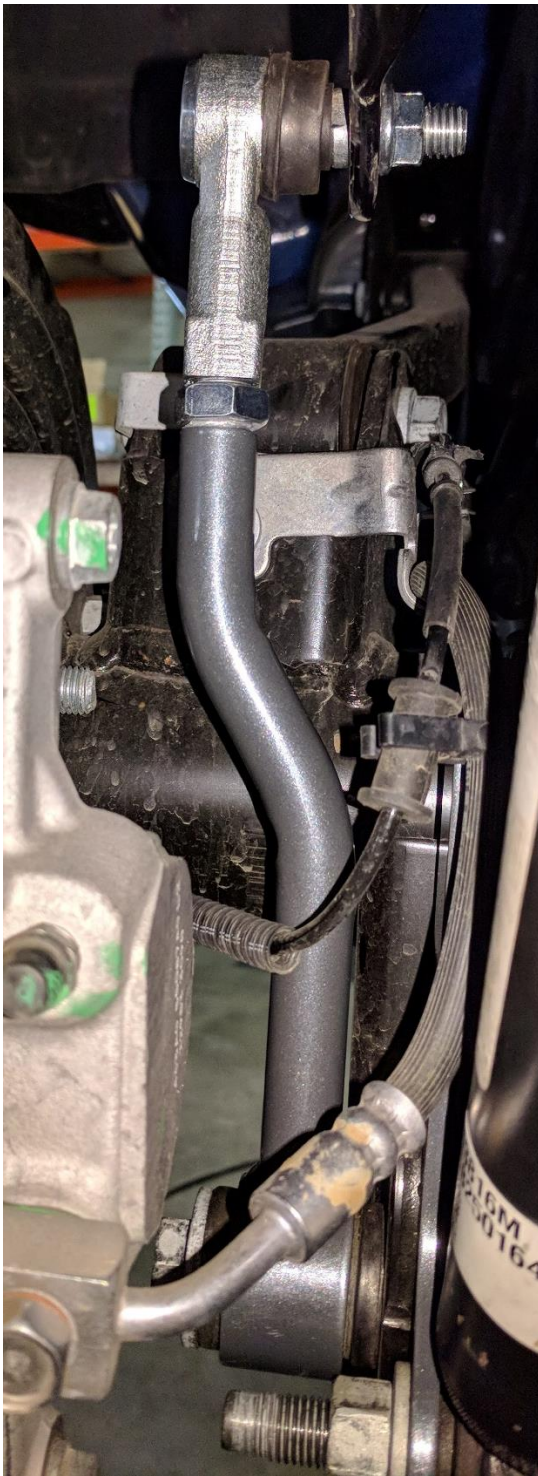
Figures 1 and 2. Correctly Installed Rear Sway Bar Links (Driver on Left, Passenger on Right)
