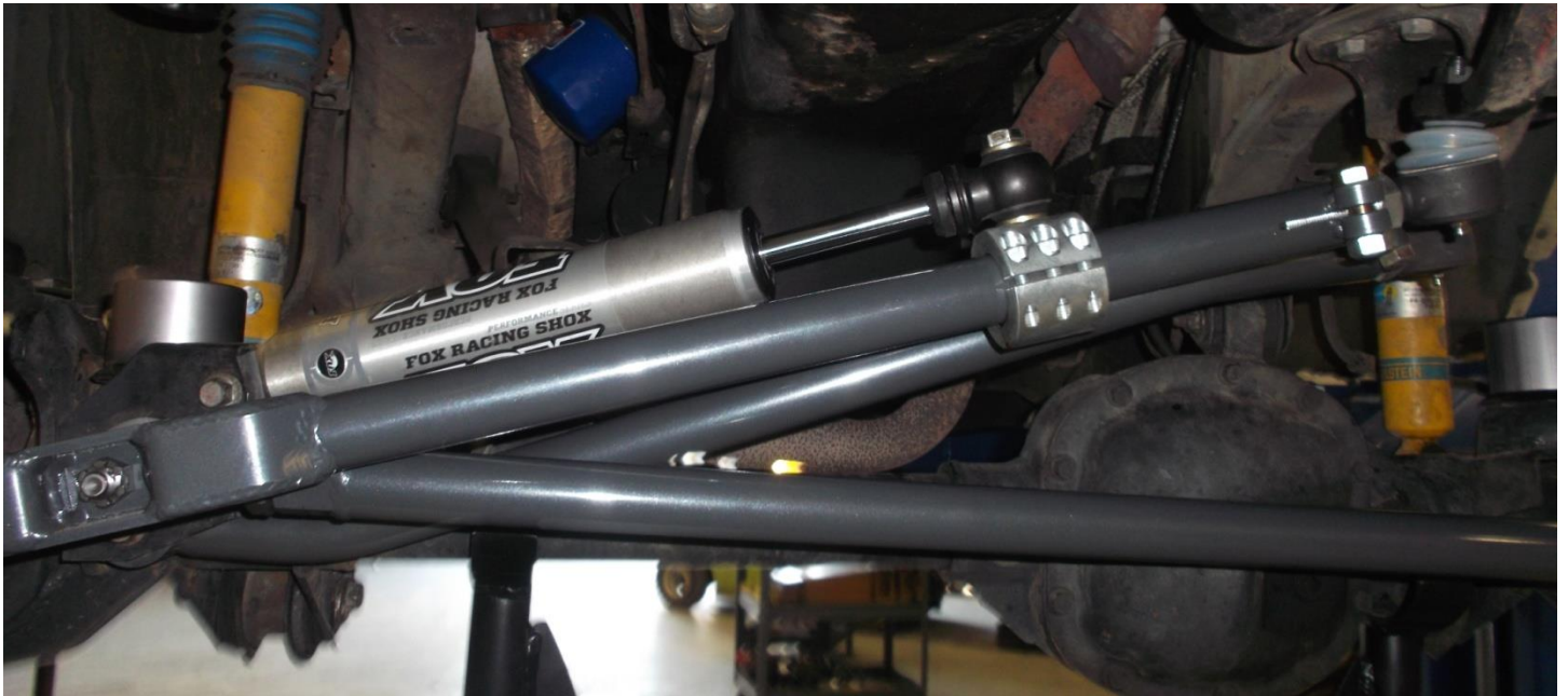
Figure 6. Correctly Installed Steering Stabilizer
