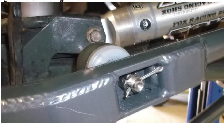
Figure 4. Cotter Pin Bent To Engage Tie Rod End Stud
