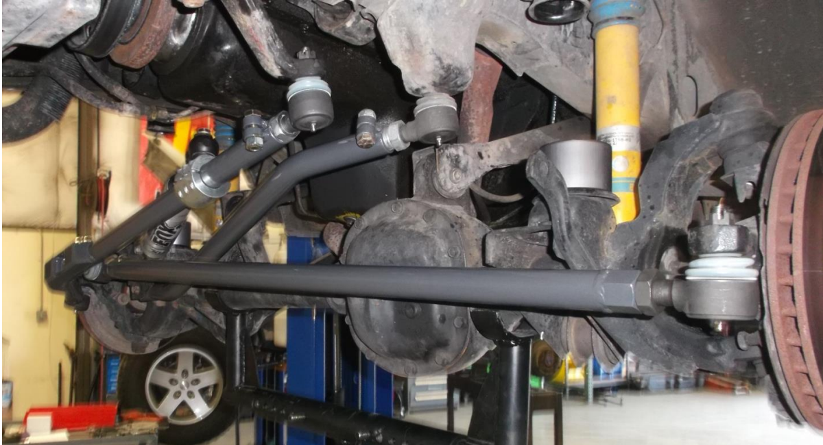
Figure 3. Synergy Tie Rod Installed
