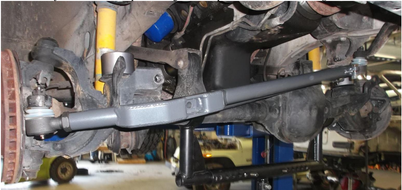
Figure 2. Synergy Drag Link Installed
