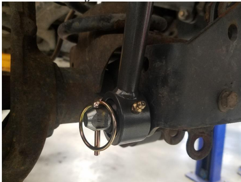
Figure 3. Sway bar bushing end with quick disconnect studs.
