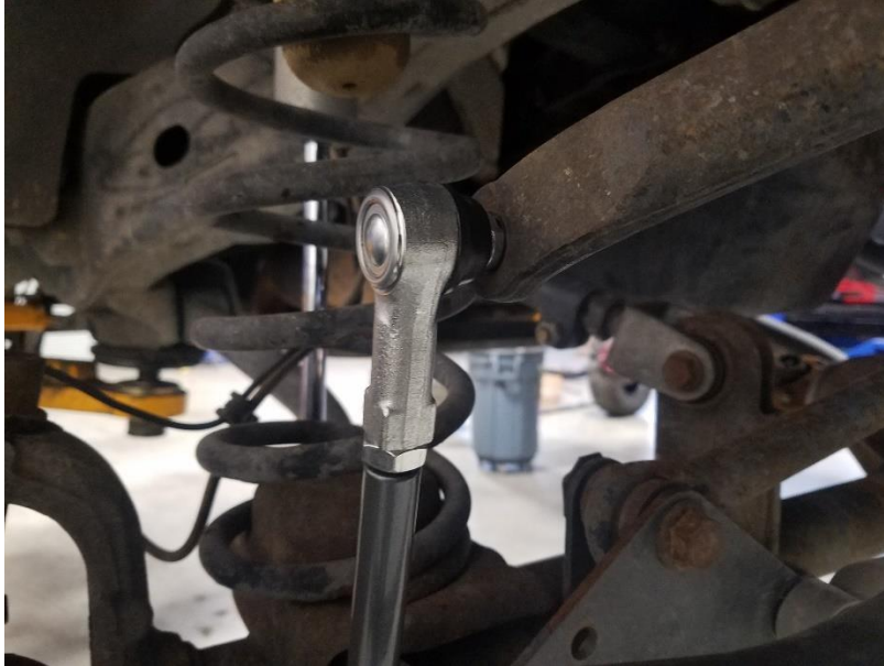
Figure 2. Correct sway bar link rod end orientation.
