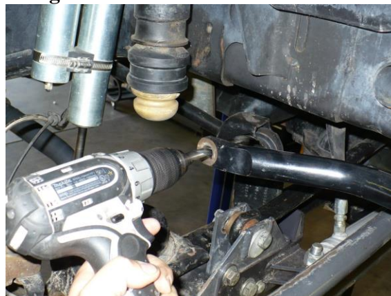
Figure 1. Drilling Out the Sway Bar
