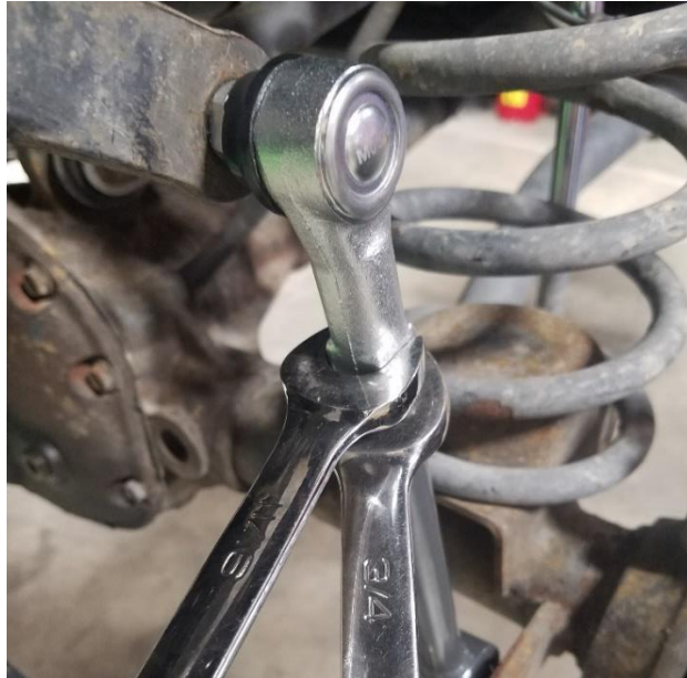
Figure 4. Tightening the tie rod end jam nut.
