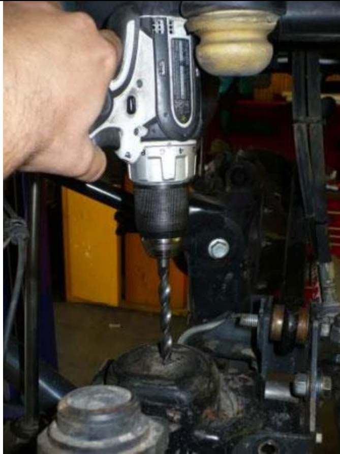
FIGURE 1. Drilling 3/8” Hole in Coil Perch/Bump Stop Pad
