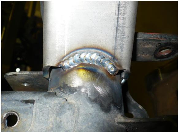
8. After welding, clean off any weld burrs and paint the desired color to prevent corrosion.
