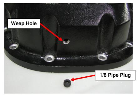
Figure 3: Weep Hole and 1/8 Pipe Plug
