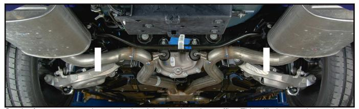
Cut the factory system close to the bend that leads to the muffler. This will give you the maximum amount of material for adjustments.
