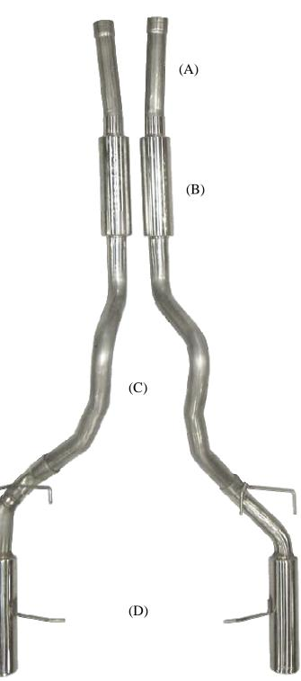
NOTE: For customers that have installed a 3" X or H pipe you must order the optional TFM62B-3 front Pipes and two HVC66 3" butt clamps if you do not already have them to make the system a direct bolt on.
