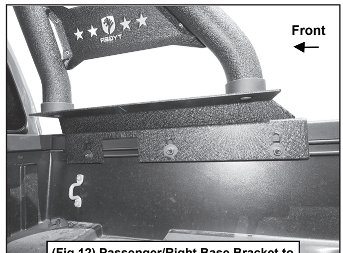
(Fig 12) Passenger/Right Base Bracket to bed installation
