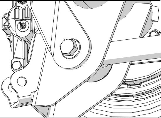
Reinstall the trackbar into the bracket using the upper hole and the factory hardware. Torque to 125 ft-lbs.
