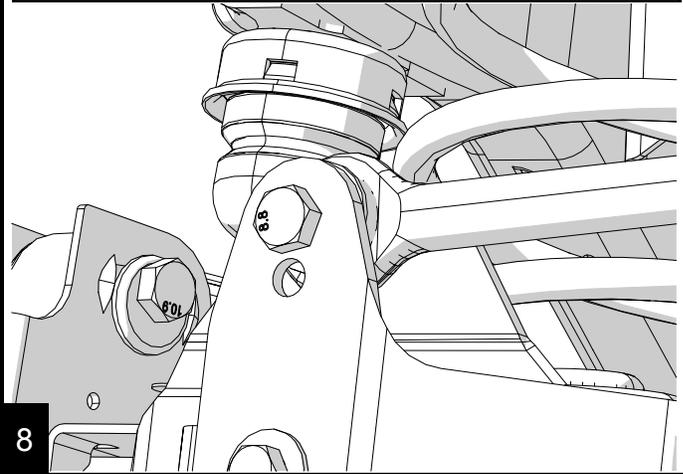
**Caution:** The trackbar bolt can rub on the rear driver side spring. To avoid this turn/clock the rear springs to where the pigtail end is to the rear of the Jeep.
