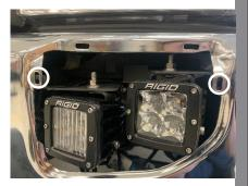
Use a 3mm hex key to for the button head and an 8mm socket to tighten the nyloc's.
