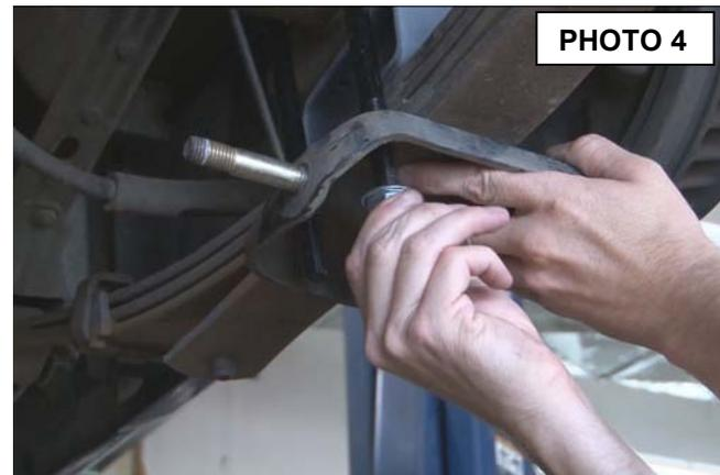
7. Install the lower mount of the rear factory shock to the u-bolt plate using factory hardware and a 21mm socket.
