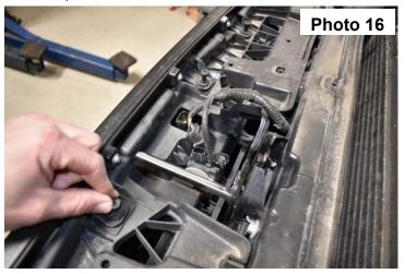
18. Reinstall the headlight trim with factory hardware and reinstall the upper radiator cover.
