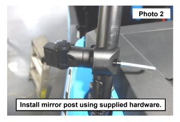
Insert the mirror into the mirror post and secure using the supplied bolts and Allen wrench.
