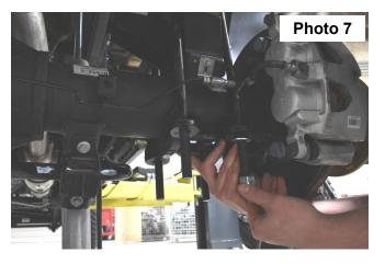
11. Locate shock part number 660805. Using an 18mm wrench, for the upper, and a 19mm and 15mm wrench for the lower. Install using factory hardware on upper and lower shock mount. Torque to 60 ft-lbs.
