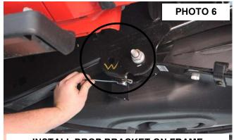
INSTALL DROP BRACKET ON FRAME
