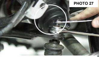
**REINSTALL THE SWAYBAR ON CONTROL ARM**
