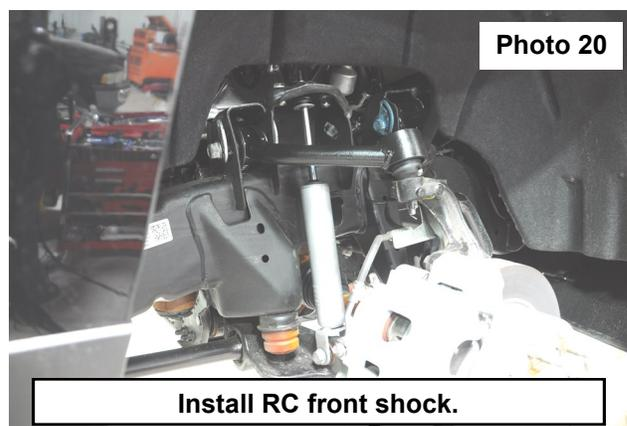
25. Install the factory lower shock hardware. Torque the upper and lower hardware to factory specs using a 21mm.
