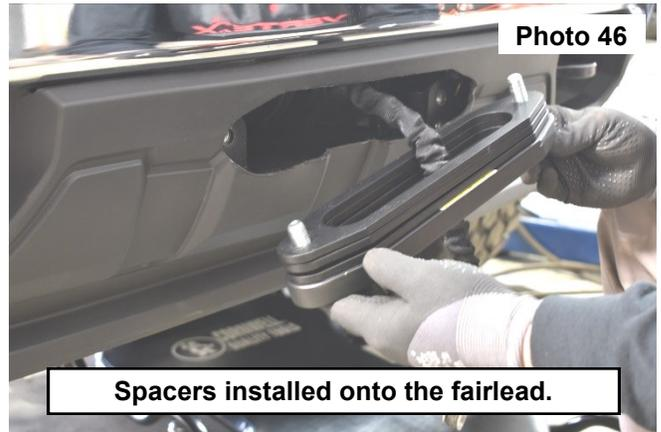
**Spacers installed onto the fairlead.**
