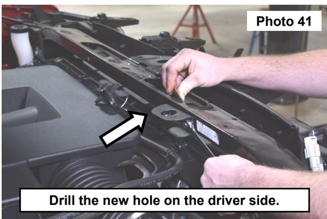
**Drill the new hole on the driver side.**
