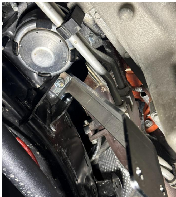
Figure 37: Motor mount bracket loosely installed
