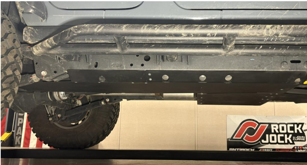
Figure 24: Gas tank skid plate fully installed
