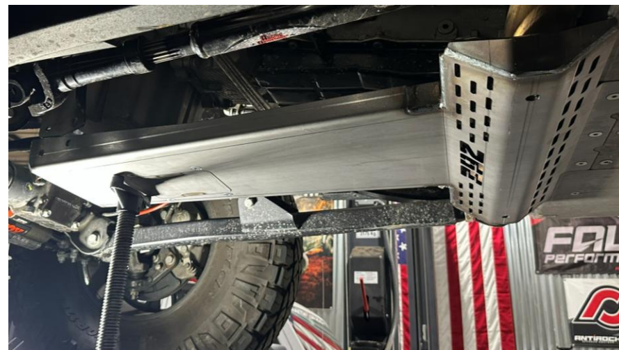
Figure 38: New skid plate installed at OEM cross member with supplied cross member components
