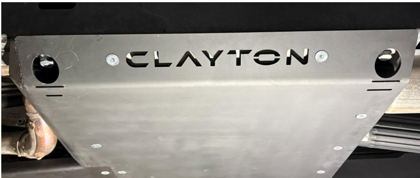
Figure 27: "CLAYTON" Logo backing plate installed (unpainted)
