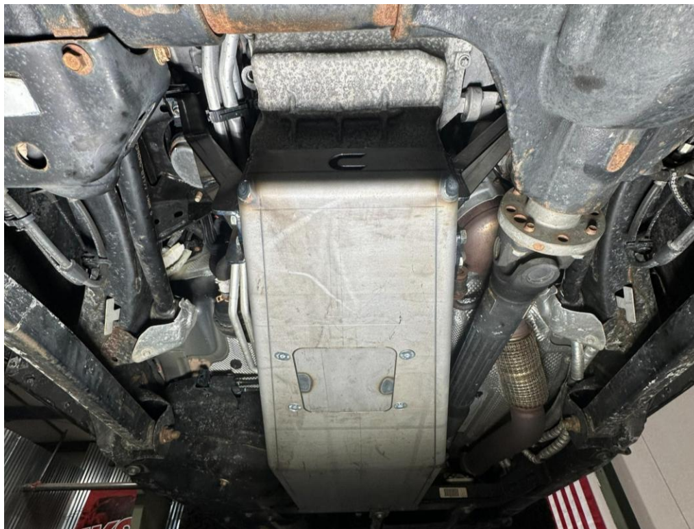
Figure 41: Engine skid plate fully installed
