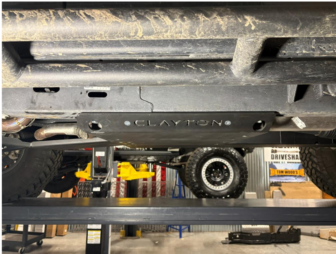
Figure 33: Transfer case skid plate fully installed
