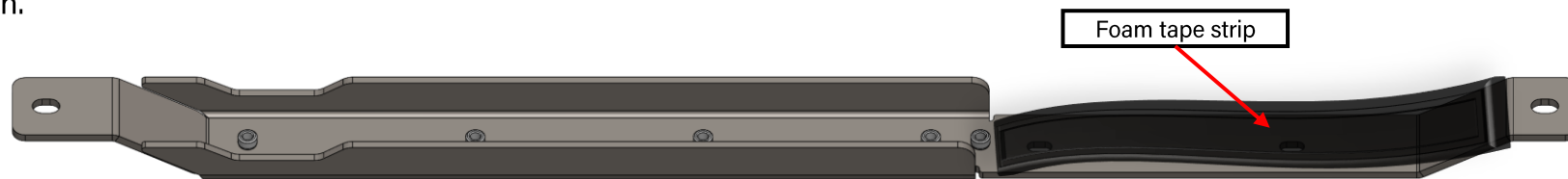
Figure 14: Skid support member with gasket tape applied
