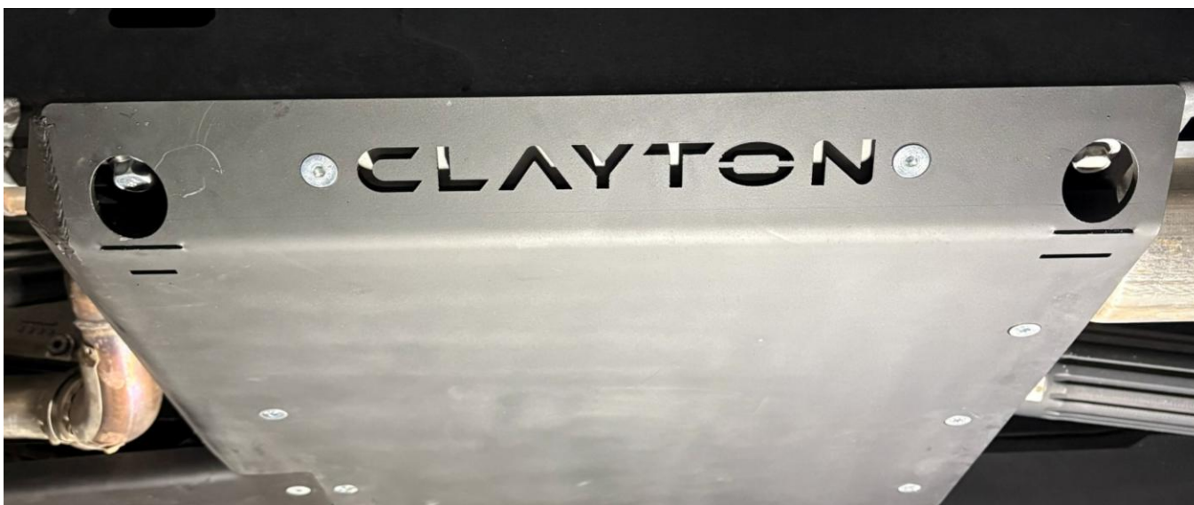
Figure 27: "CLAYTON" Logo backing plate installed (unpainted)
