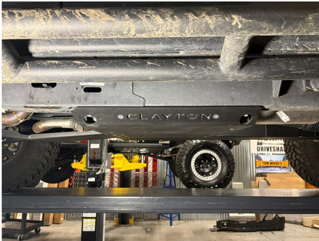
Figure 33: Transfer case skid plate fully installed
