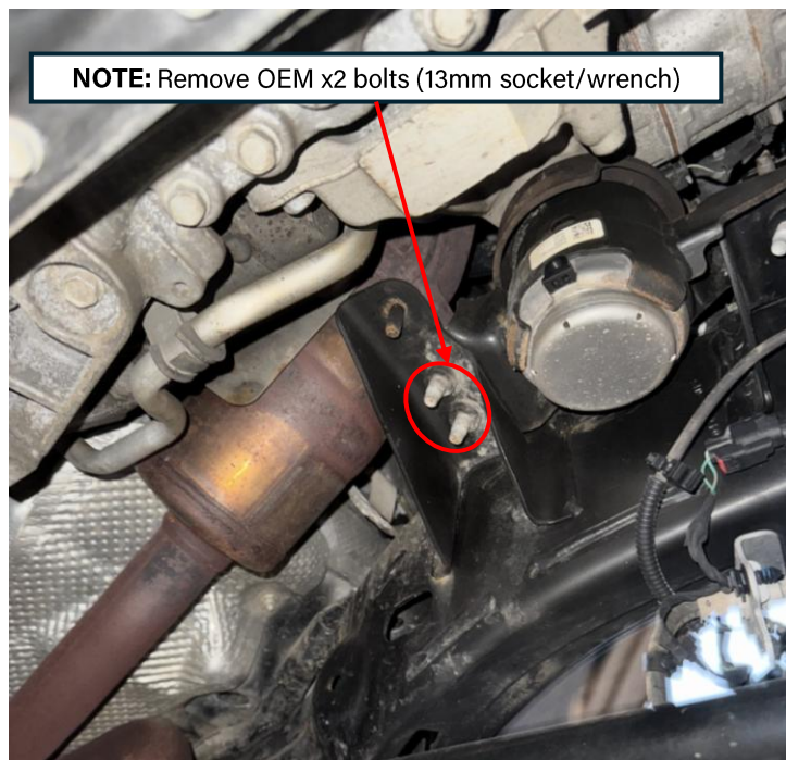
Figure 34: Motor mount old/new bolts with CAD visual showing bolt swap
