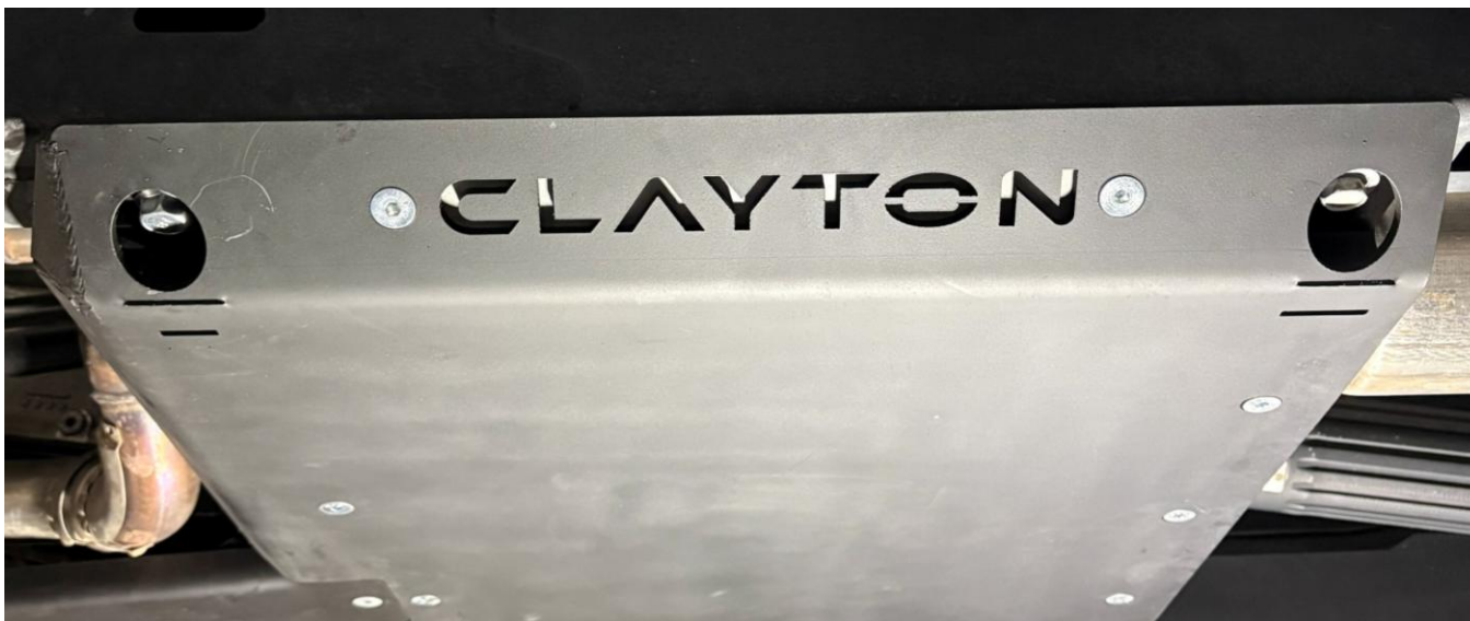
Figure 27: "CLAYTON" Logo backing plate installed (unpainted)
