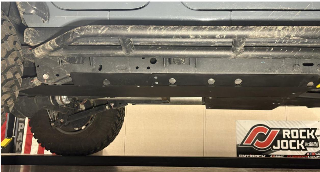
Figure 24: Gas tank skid plate fully installed
