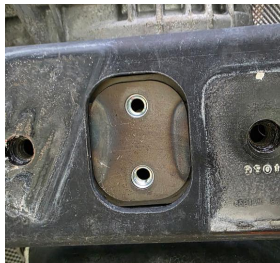
Figure 26: Installing cross-member components (Aluminum cross member)
