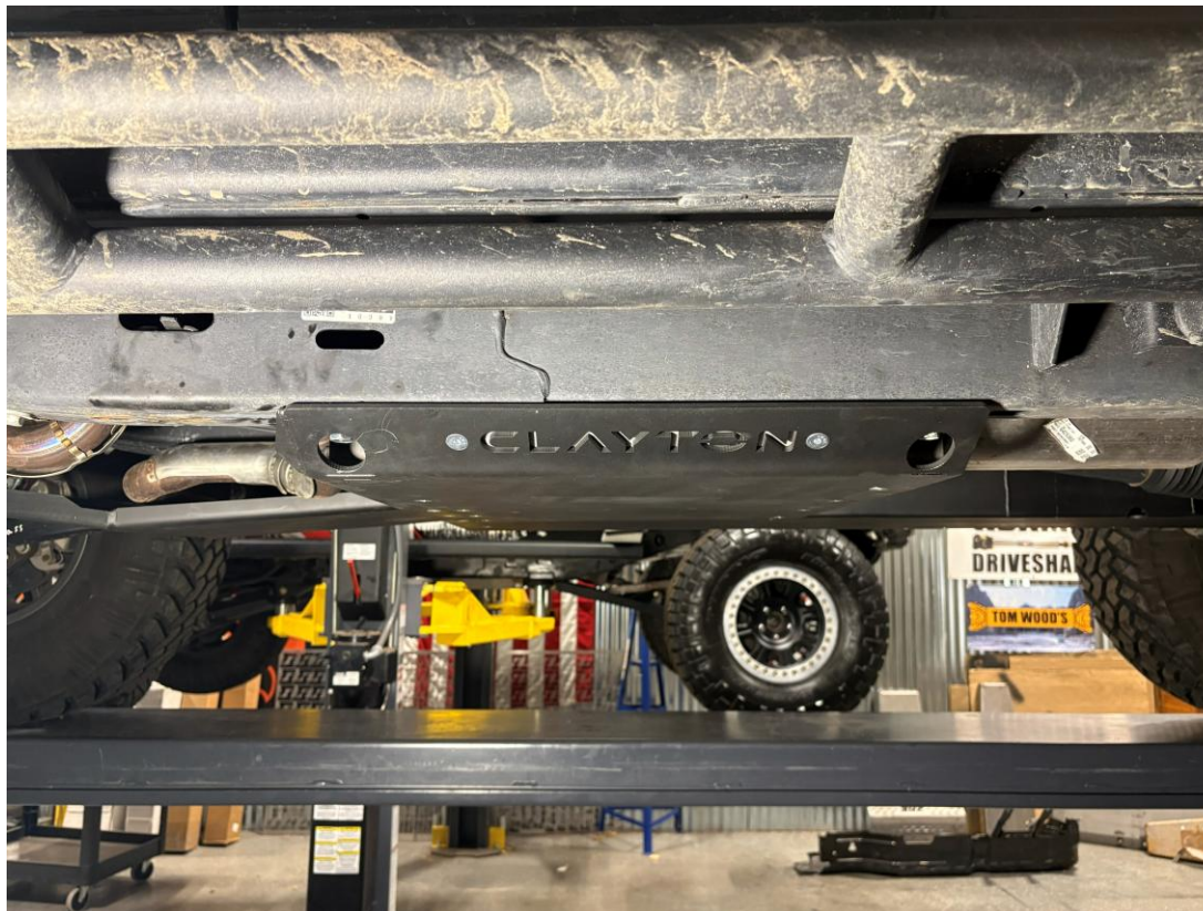
Figure 33: Transfer case skid plate fully installed
