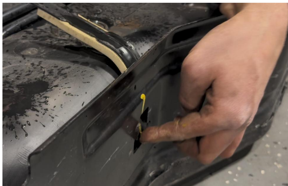
Figure 12: OEM tank strap removal
