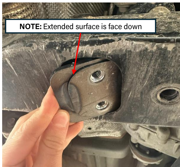
Figure 25: Installing cross-member components (Steel cross member)
