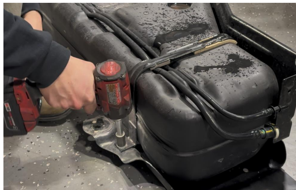
Figure 12: OEM tank strap removal
