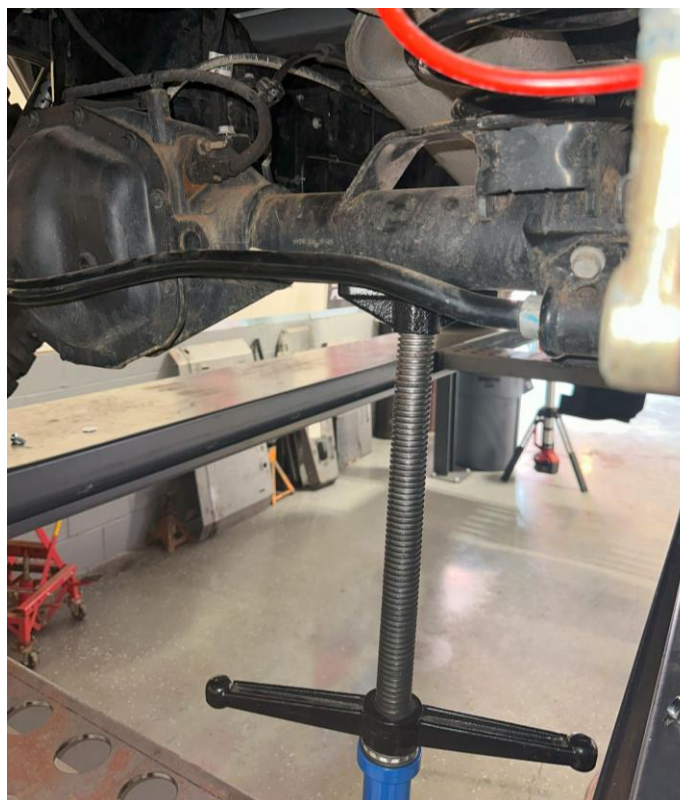
Figure 1: Vehicle positioned on a four-post lift with supporting axle jack stand
