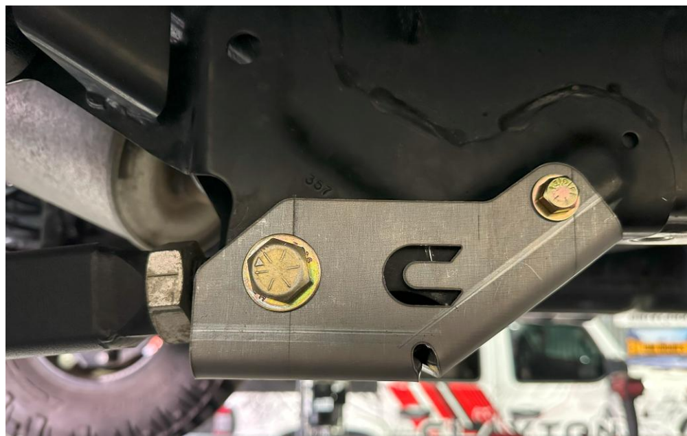
Figure 9: Prototype (unpainted) skid plate torqued to specification
