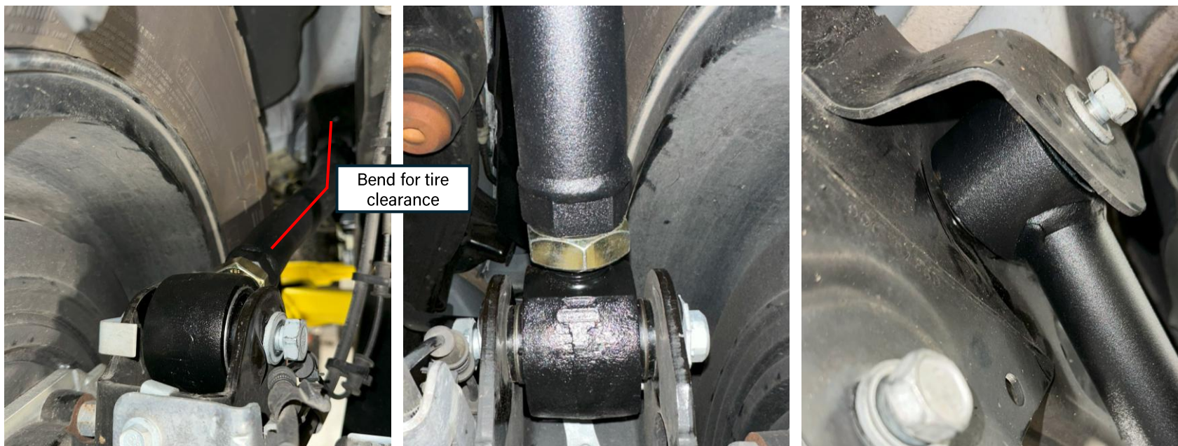
1709103 (OVERLAND+ Series) Rear upper control arm installed
