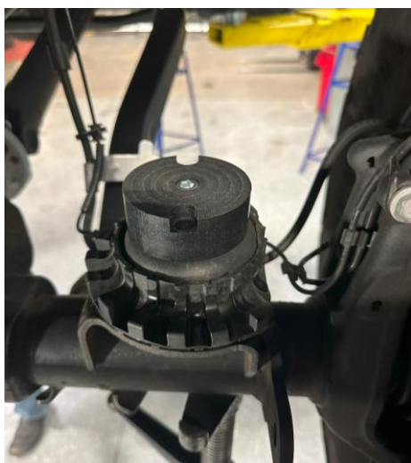
Figure 2: Bump stop installed on front 2018+ JL axle
