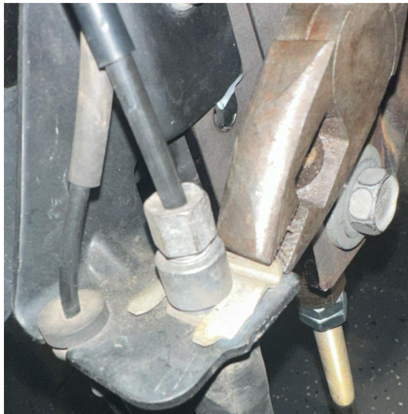
Removing the brake line retaining clip
