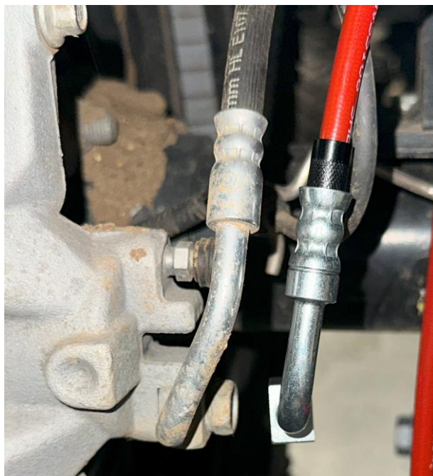
Proper Banjo Fitting orientation (rear driver's side)
