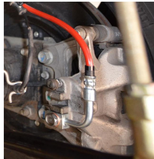
New banjo fitting installed (rear passenger's side)
