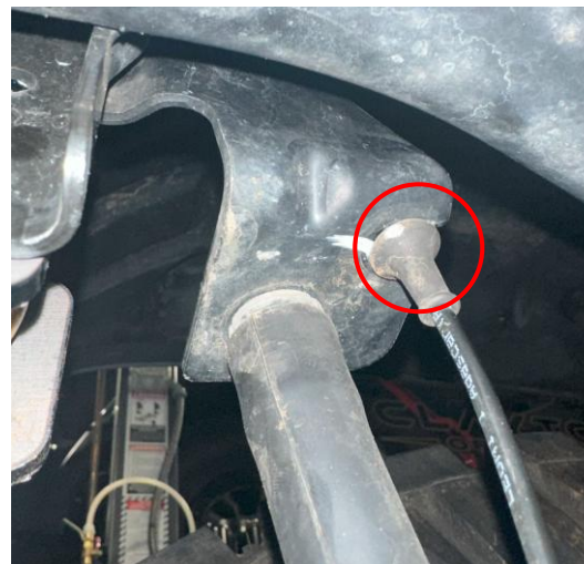
Frame mount ABS cable to be removed
