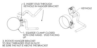
3. Install the **Muffler** onto the **Front Pipe** using the **Hang Tight<sup>™</sup> Hanger** from step 2.
