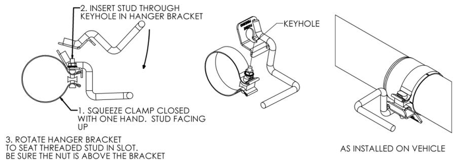
2. On Quad Cab Short Box, and Regular Cab Long Box models, install the expanded end of the **Extension Pipe** over the factory exhaust system behind the "Y" pipe using a **3" Clamp**.
